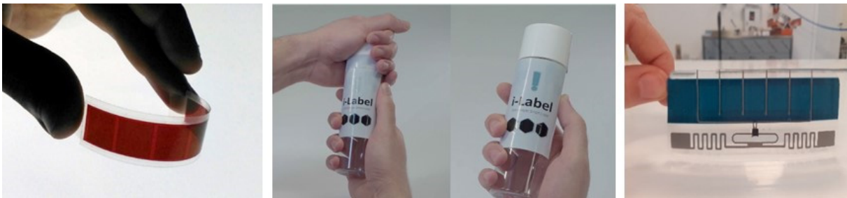
Figure IV-8. Flexible PV device produced by Ribes Tech as indoor light harvester (left), fully printed prototype of an anti-tampering label self-powered by indoor light (courtesy of Ribes Tech) (center) and active UHF electronic label composed of an IC coupled to a PV harvester, and printed on the same substrate: the device is the result of a joint development done by Ribes Tech and Lab-ID (right).
