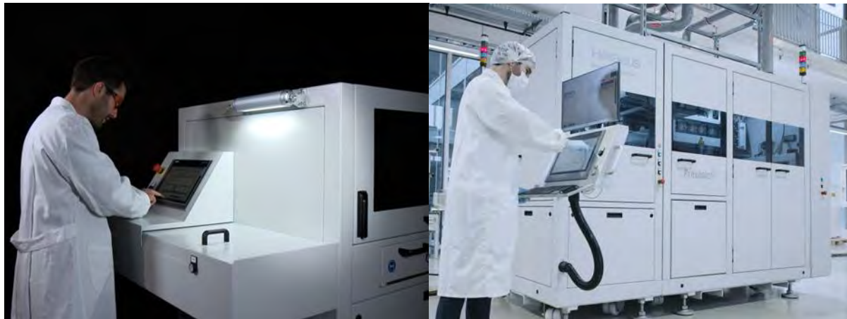
Figure 4.1.2: Upscaling of inkjet printing equipment to realize the upscale from lab based prototyping to mass production equipment suited for semiconductor industry (Heraeus Prexonics System solution). (3)
