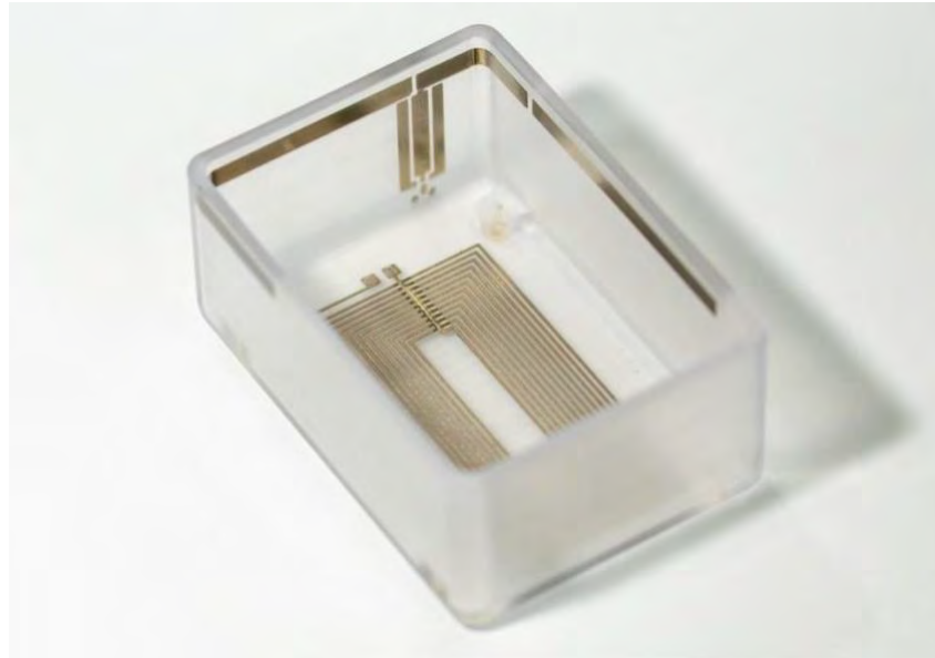
Fig. 2.6.4. Ag nanoparticle antenna Aerosol Jet printed inside an injection molded PC body. Courtesy University Erlangen Nuremberg - FAPS Institute
