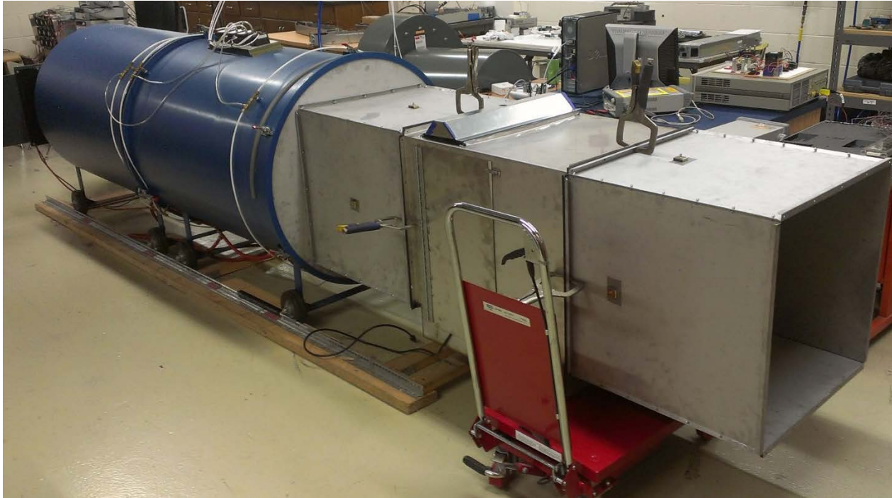
Cooling pad test duct attached to an airflow bench
