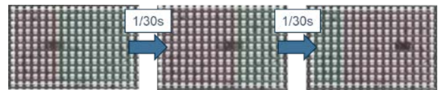
Figure 14. Long range particle motion. Particle is measured moving multiple electrodes over a single video frame with an average velocity of 6 mm/s. Chip is 50 \mu\text{m} x 100 \mu\text{m} . The actuator grid pitch is 50 \mu\text{m} . Ref: Rupp (SID 2021)
