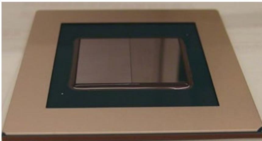
Figure 14: Chiplets integration through InFO technology for networking
