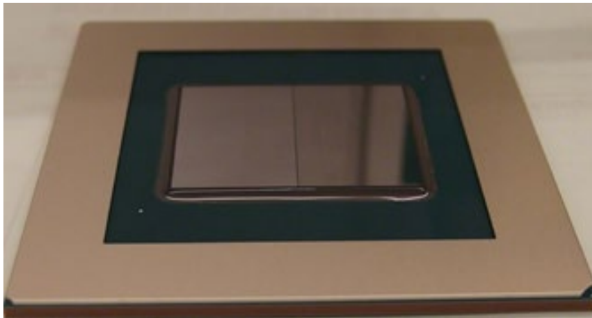
Figure 14: Chiplets integration through InFO technology for networking
