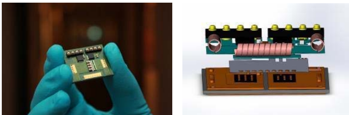
Figure 14. Example of EMI-optimized SiP SiC Module. Source: Fraunhofer IZM
