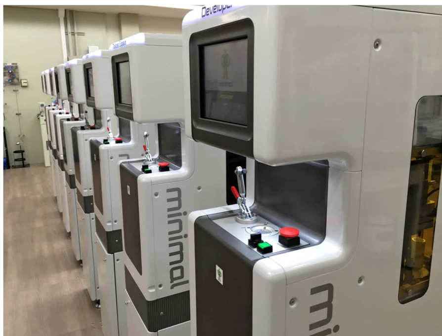
Figure 9-3. Minimal modular wafer fabrication technology
