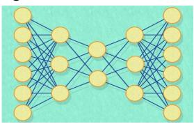
A machine-learning system analyzes materials "recipes" using an autoencoder. If successfully trained, the system will capture the data's characteristics.
