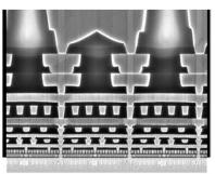
Cobalt & Cobalt/Copper, in use today. Contact resistance reduced 1.5X, Line resistance down 60%. Intel
