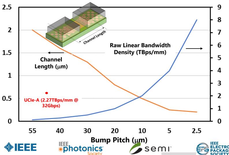
@ 32Gbps UCle-A theoretical BW@ 45µm pitch is 2.2716 TBps & this roadmap states @ 3Gbps & @ 40µm pitch a theoretical BW of 0.25TBps is possible. There is no discrepancy in the numbers and modulating speed (hence power efficiency) is a knob for scaling BW  $\rightarrow$  lots of room to grow
