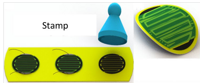
(e) gravure printed super capacitor
