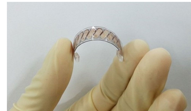
Wearable TEG: KAIST, 40mW @ wristband size
