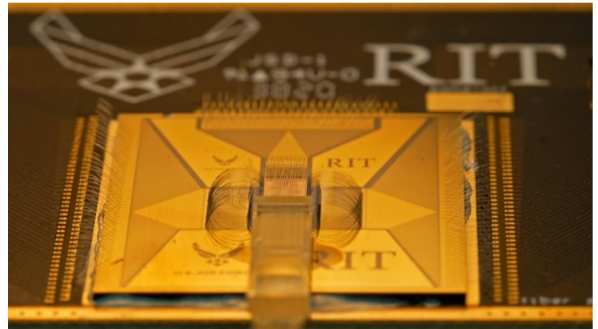
Fig. 2. Packaged quantum photonic processor QPIC with hundreds of electrical wirebonds and a fiber array attached to the QPIC. (S. Preble, RIT)
