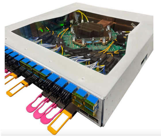
Figure 10 Cisco’s 25.6T CPO System demonstrated in OFC 2023
