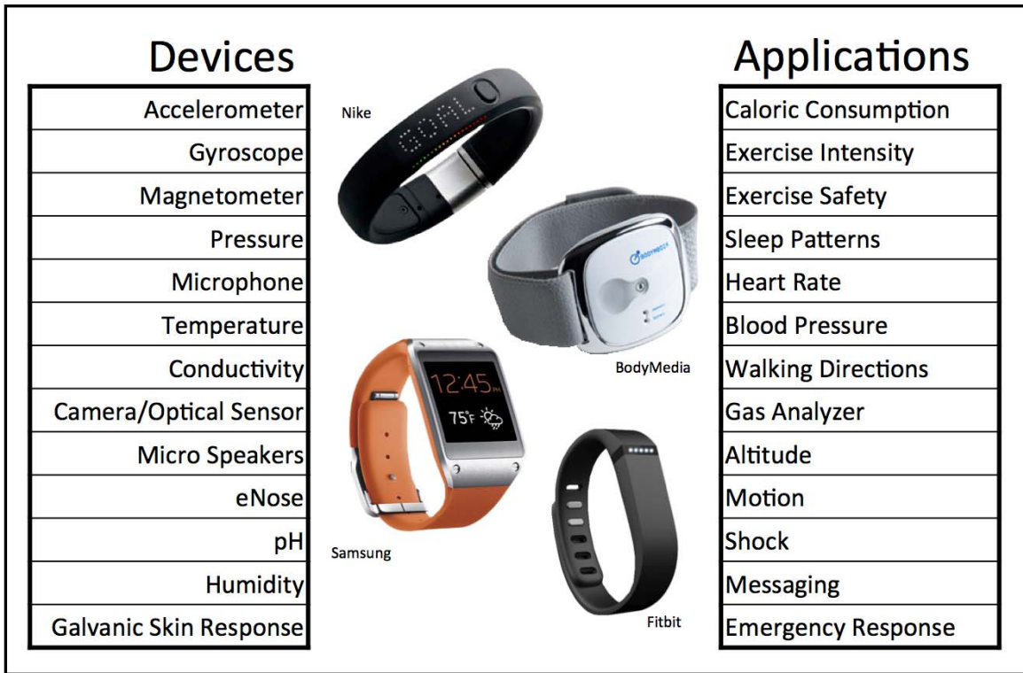
Figure 4 Sensors trends for “Wearable” technologies. The column on the left lists the types of sensors that are already in or may be added to wearable devices, and the column on the right lists the types of functions are already or may be added using these sensors.
