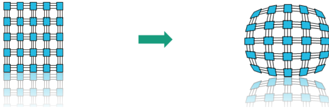
Fig. 5: Schematic for the structure and behavior of the stretchable circuit board.
