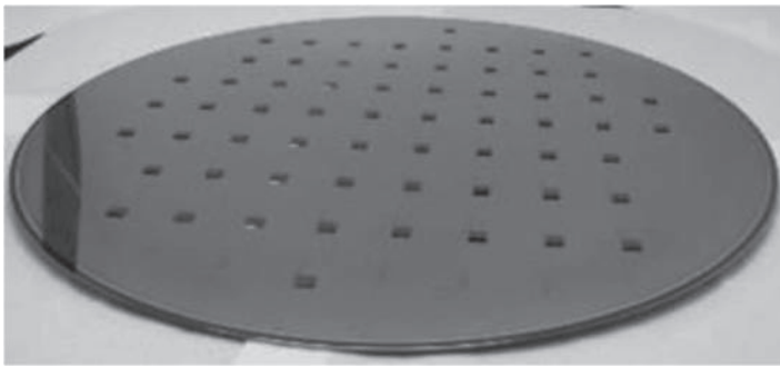
Figure 10: Chip-to-Wafer Hybrid Bonding integration
