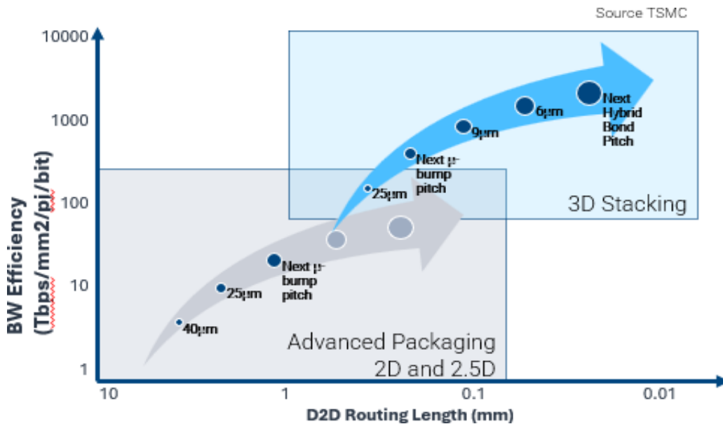
Figure 13.7.2: Illustrative Bump Pitch Scaling Trend in 2.5D and 3D Packages.
